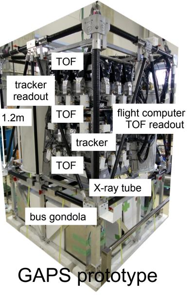
• GAPS prototype flight in 2012 met 100% of its goals and demonstrated all key technologies Si(Li) detector fabrication well understood
